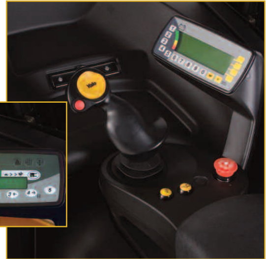
Side-stance control handle with optional premium display (Inset Photo: standard display)
