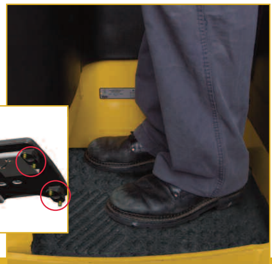
E-Z Ride floor with elastomeric mounts
