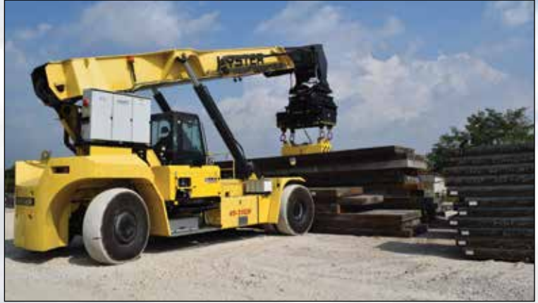
Versatility is key for the RS46 series. Magnet attachment for handling steel slabs shown.
