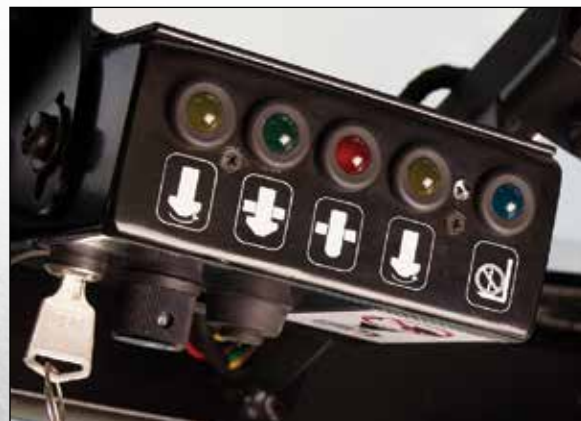
Twistlock module with indicator lights
