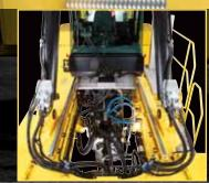
THE EASILY REMOVABLE TOP DECK PLATES WITH QUICK DISCONNECT LATCHES PROVIDES FAST ACCESS TO MAJOR COMPONENTS.
