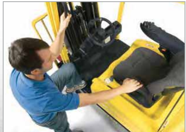
Three-point entry into operator compartment
